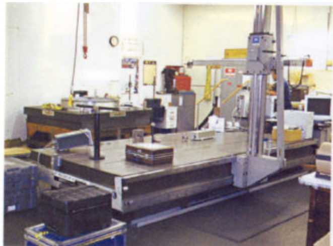
View of the MCV 4000 checking Z-axis motion on the Brown & Sharpe CMM. A mirror attachment is used for the purpose.
