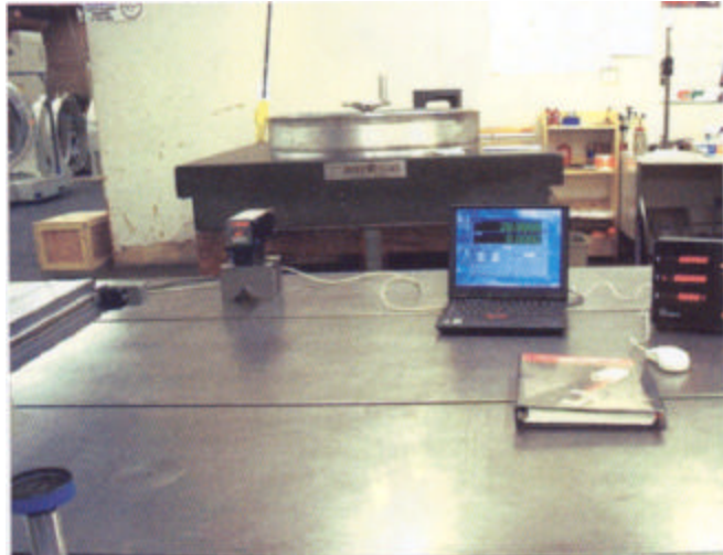
Data collection during calibration of Tapemations's large Brown and Sharpe MDL 3000 Validator CUM. The MCV 4000 laser head is shown at the left-rear corner of the CMM tabletop. Laptop stores data.
