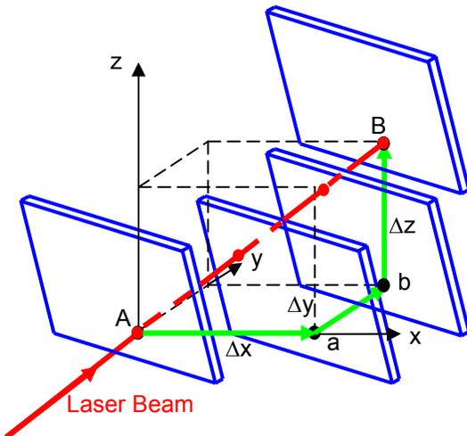
LaserVector 2: The laser vector measurement technique
