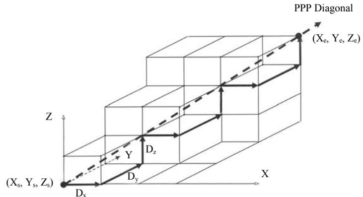
LaserVector 1: The vector measurement is pointing in the ppp diagonal direction. Move  $D_x$ , stop, collect data, move  $D_y$ , stop and, move  $D_z$ , stop, collect data and so on.
