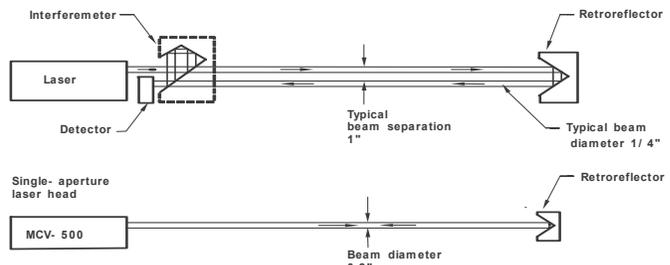
Fig. 1 A comparison of a laser interferometer and a single-aperture Laser Doppler system
