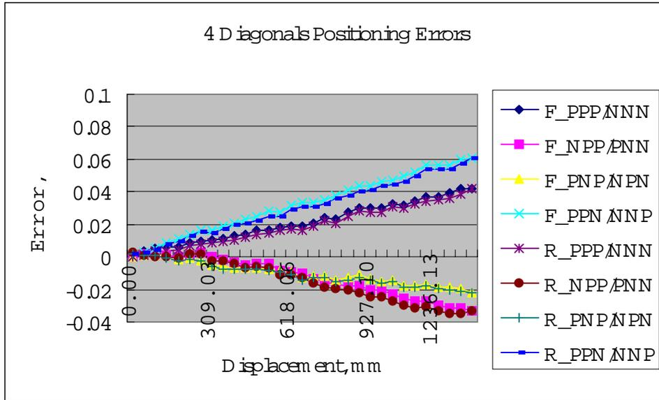
7. Four body diagonal displacement errors measured with pitch error compensation. The total error is 95  $\mu\text{m}$ . A small improvement.
