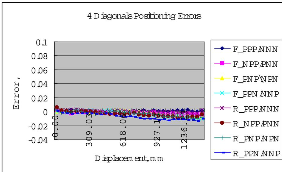
8. Four body diagonal displacement errors measured with pitch error and straightness error compensation. The total error is 16  $\mu\text{m}$ . An improvement of 700%.
