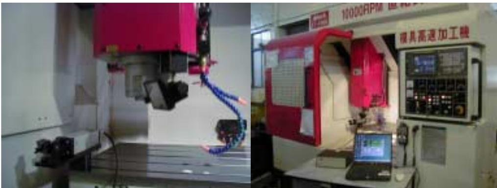
2. A photo of the AWEA vertical machining center and the sequential diagonal measurement setup with the laser on the table and the flat mirror on the spindle.
