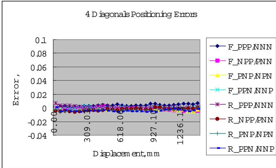
9. Four body diagonal displacement errors measured with volumetric compensation. The total error is 12.5  $\mu\text{m}$ . An improvement of 900%.
