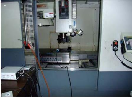
Fig.6: Laser vector step diagonal measurement
