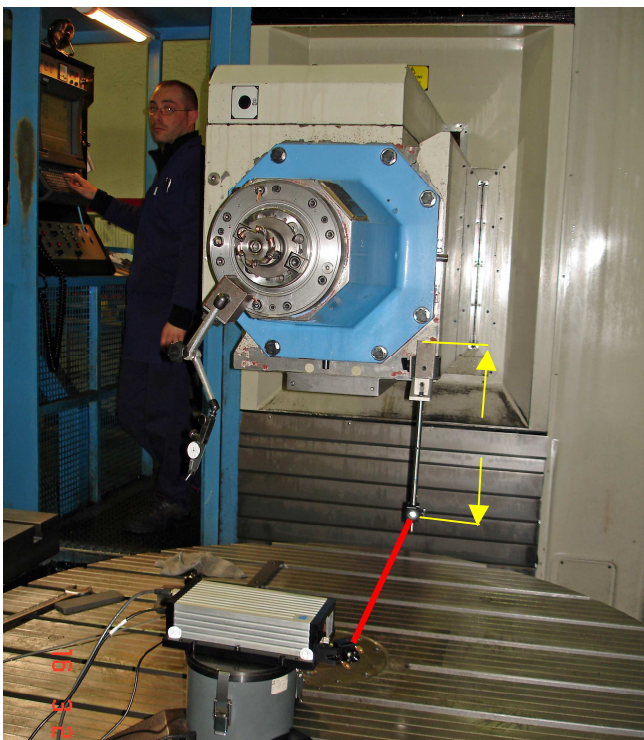
Fig.6 Measurement of positioning accuracy with retroreflector outreach. The laser his in the position Low, while the machine is in the position High. The retroreflector is connected with a spacer bar to the RAM.
