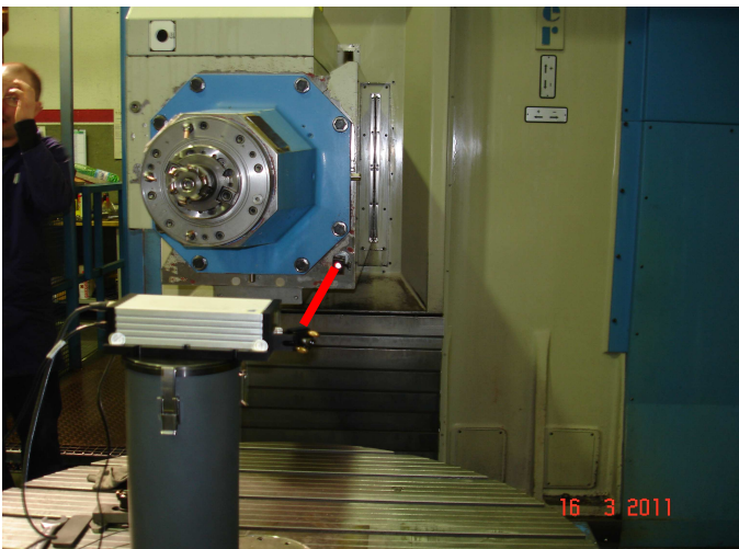
Fig.1 Measurement of the position error in the Position High, both the laser than the axis are in the higher Y position.
