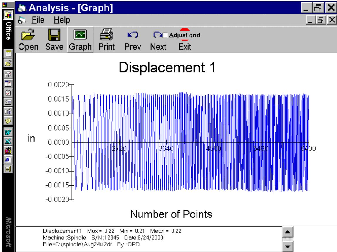
Fig. 3 Spindle run-out at various speeds from 500 to 2500 RPM
