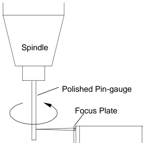
Fig. 2 Non-contact measurement of spindle runout
