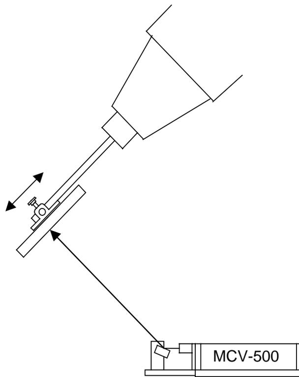
Fig. 1 Non-contact measurement of rotational angle of a 5-axis machine
