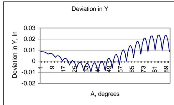
Fig. 3, Measured deviations in Y-direction due to the angular errors
