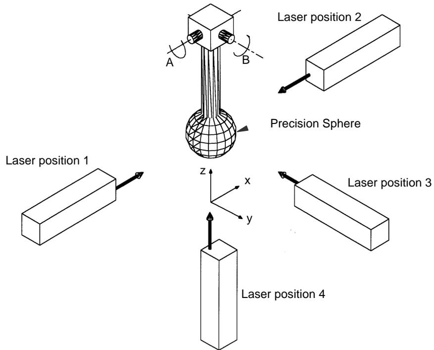
Fig. 1, Schematics of a 5-axis spindle with a precision sphere and laser positions
