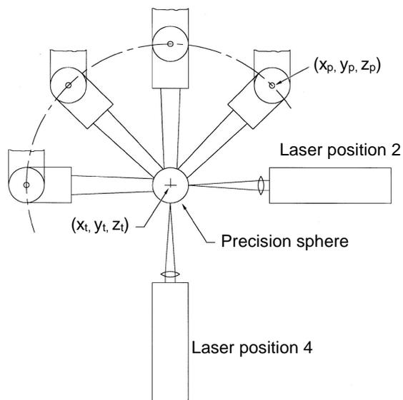
Fig. 2, Schematics of a 5-axis motion with the center of the precision sphere at a fixed position
