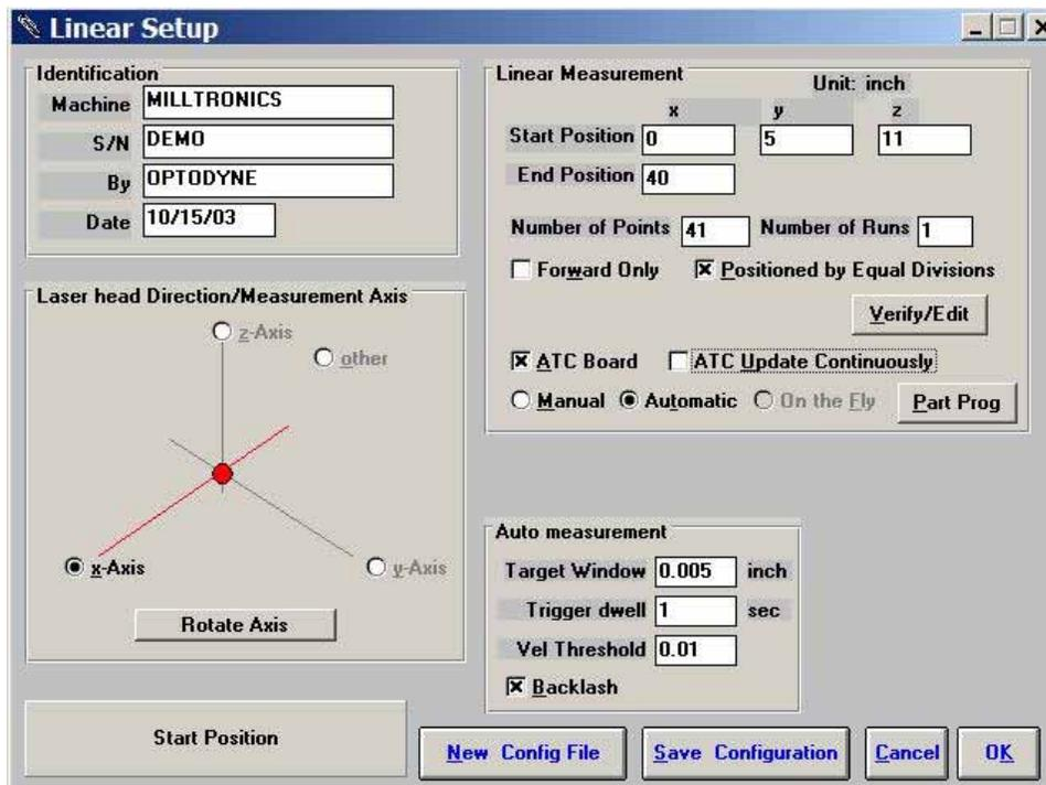
Fig. 1, A popup screen for user to enter the location of the laser beam.
