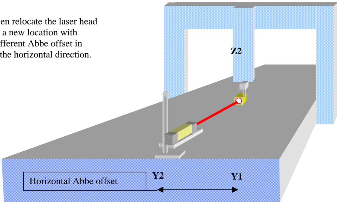
Fig3 Example of laser position at the second measurement
