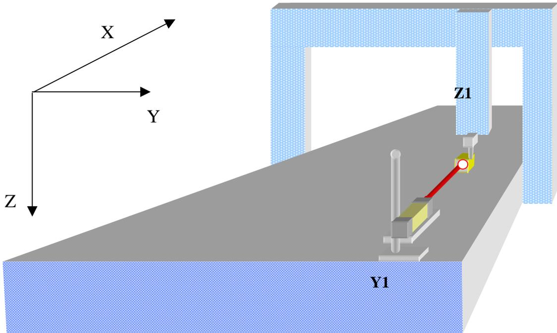
Fig2 Example of laser position at the first measurement
