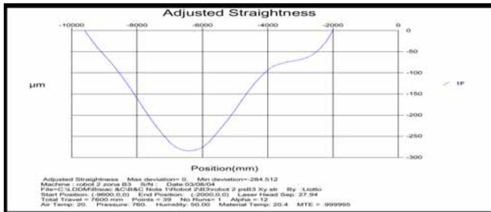
Fig. 6, A vertical straightness analyzed and calculated by LDDM software
