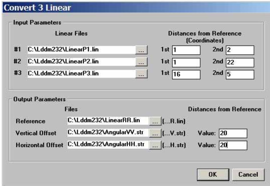
Fig. 5, A Popup Screen for User to Enter 3 Linear Displacement Files with Different Abbe Offsets and 3 Output File Names with 2 Different Abbe Offsets
