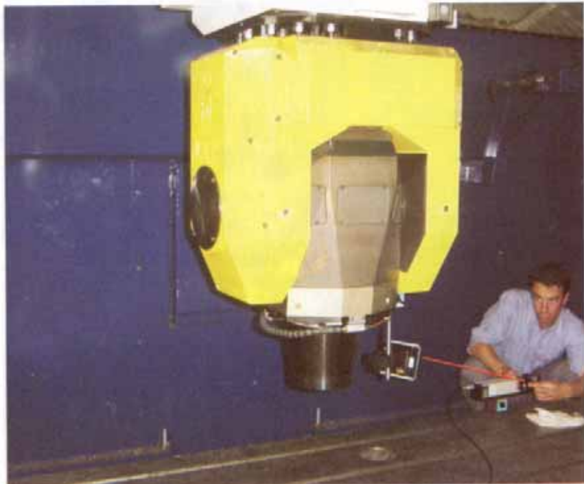
Jobs S.p.A. uses Optodyne's patented volumetric laser calibration technology on its five-axis high-speed machining centers.
