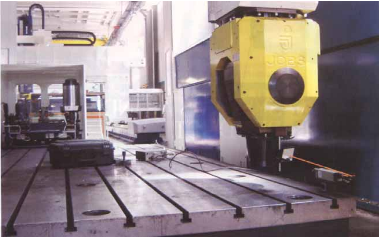
Sequential step-diagonal measurement technique collects 12 sets of data with the same four diagonal setups from which all three displacement errors, six straightness errors, and three squareness errors can be determined.
