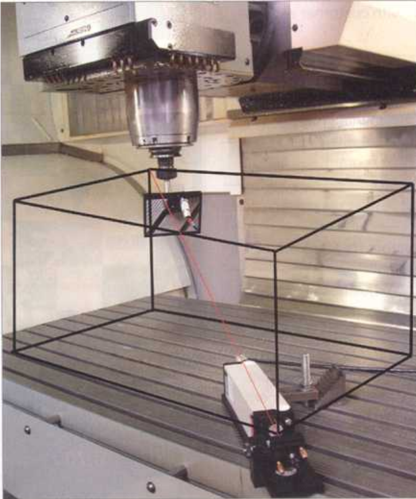
A cutting tool in a machine's spindle would trace/follow a cube-shaped path during sequential step diagonal measuring for 3D volumetric errors.
