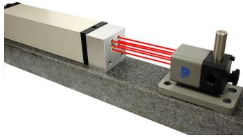
Fig. 1: Photograph of a 6-pass optical arrangement.
