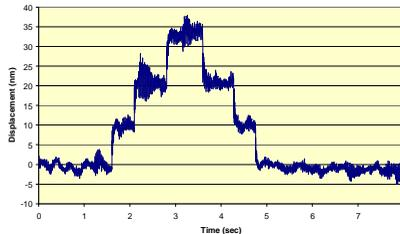
Fig. 3: Open-loop 10-nm-steps measured by the new LDDM system with single-pass optics.
