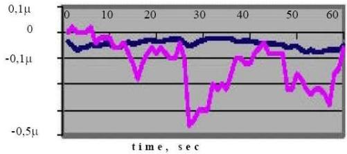
Fig. 2: Effect of air circulation on a 6-pass optical arrangement versus a single pass optical arrangement.
