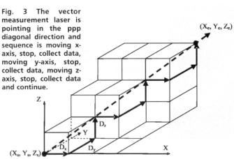
diagonal displacement measurement in that each axis moves separately in sequence and the diagonal positioning error is collected after each separate movement of the X-axis, Y-axis, and then Z-axis. This collects three times the amount of data and allows the positioning error for each separate axis movement to be measured.
