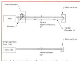
Fig. 1 A comparison of a laser interferometer and a single-aperture Laser Doppler system
