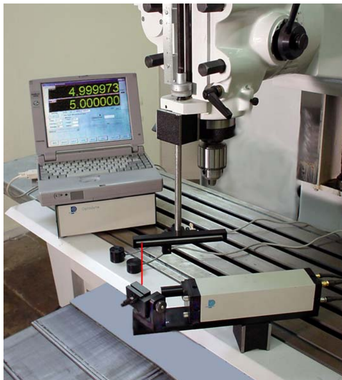
FIG. 8-2 LASER/BALLBAR CIRCULAR TEST SETUP
