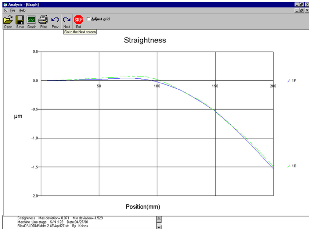
FIG. 12-9 STRAIGHTNESS PLOT, VERTICAL DEVIATIONS IN INCHES vs. POSITION
