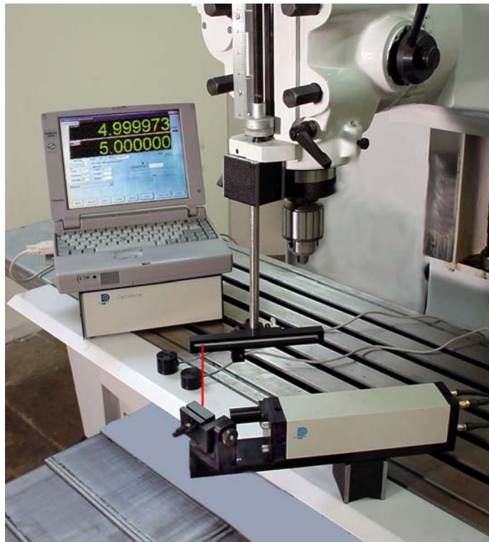
FIG. 8-2 LASER/BALLBAR CIRCULAR TEST SETUP
