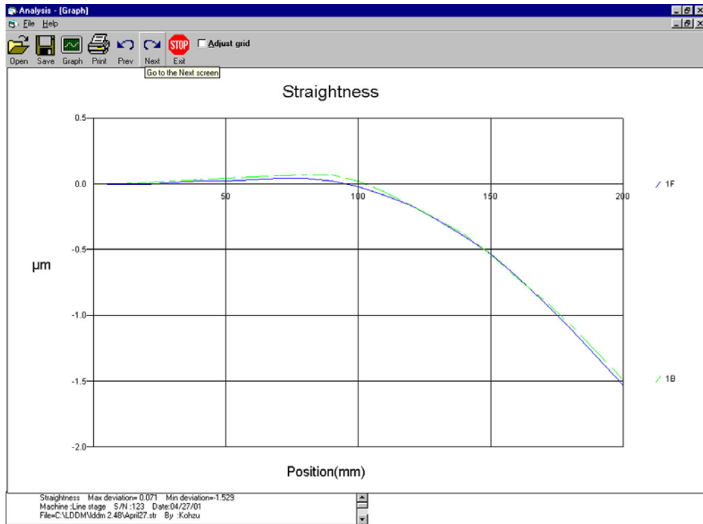
FIG. 8-9 STRAIGHTNESS PLOT, VERTICAL DEVIATIONS IN INCHES vs. POSITION
