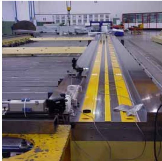
Fig. 2, Setup of a laser head and dual-retroreflector on a long guide way.
