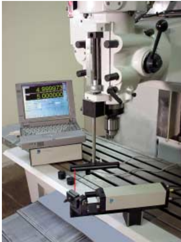
Fig. 1 A typical laser setup for the non- circular contouring measurement
