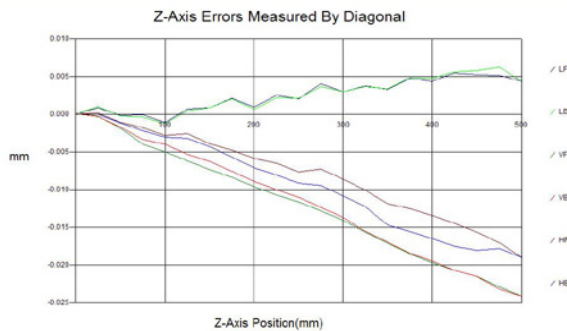
Fig 2c, Measured volumetric positioning errors of Z-axis, top traces are displacement errors, middle traces are vertical straightness errors and lower traces are horizontal straightness errors.
