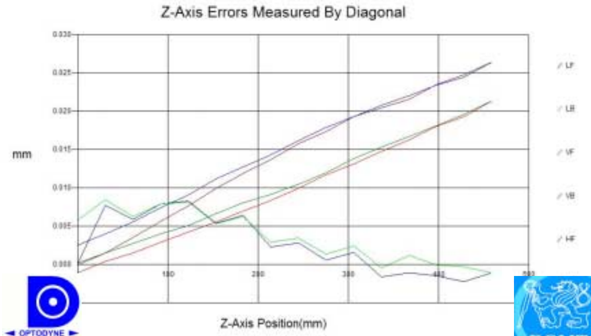
Fig. 5c Without compensation, the measured Z-axis displacement error, vertical straightness error and horizontal straightness error.
