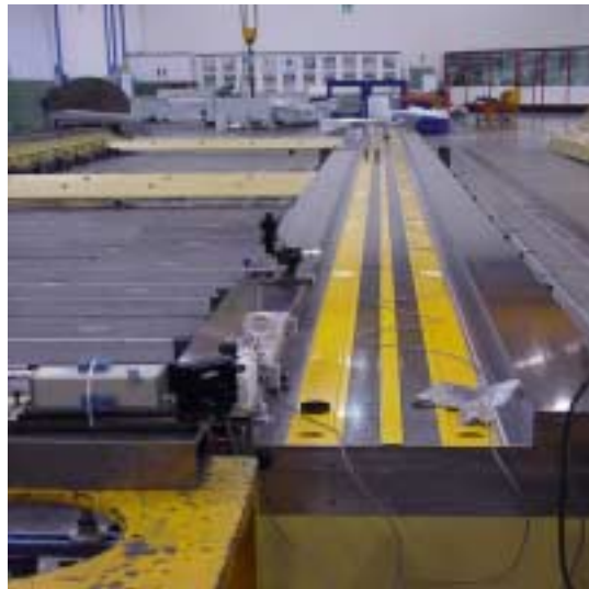
Fig. 2, Setup of a laser head and dual-retroreflector on a long guide way.
