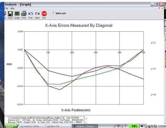
Fig. 5, Measured X-axis errors, LF, VF and HF are the displacement error, vertical straightness and Horizontal straightness, respectively.
