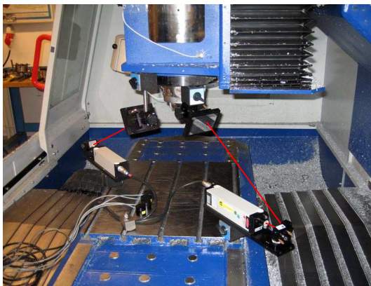
Fig. 4, A photo of the machining center and the vector measurement setup. Two lasers are mounted on the machine bed and 2 flat mirrors are mounted on the spindle.
