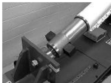
Figure 4. Lateral Transfer Hollow Retroreflector (LTHR) installed horizontally on the Hexapod Test Strut.
