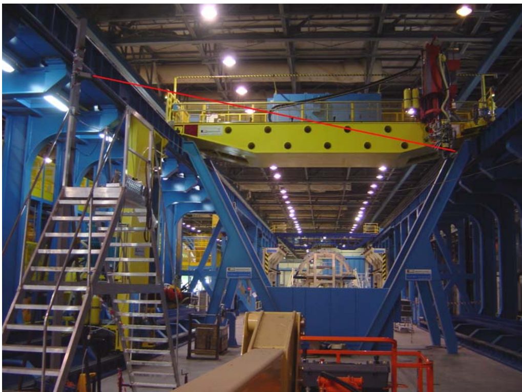
Fig. 4 : Measurement of diagonal volumetric positioning on Portal R4
