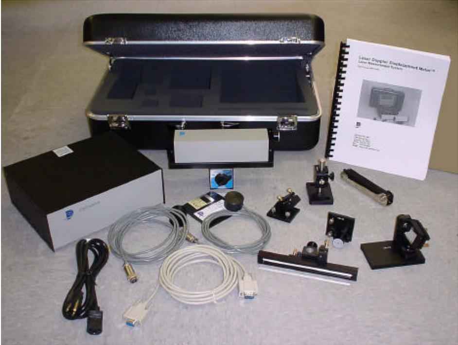
FIG. 8-1 HARDWARE FOR LASER/BALLBAR
