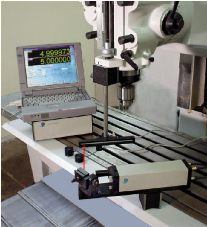
FIG. 8-2 LASER/BALLAR CIRCULAR TEST SETUP
