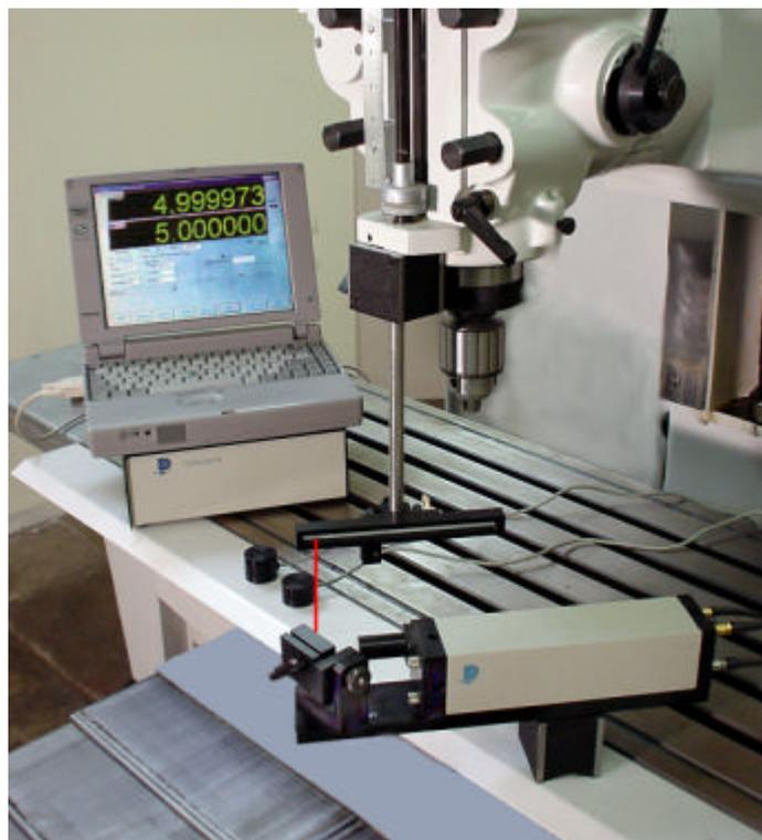
FIG. 8-2 LASER/BALLBAR CIRCULAR TEST SETUP
